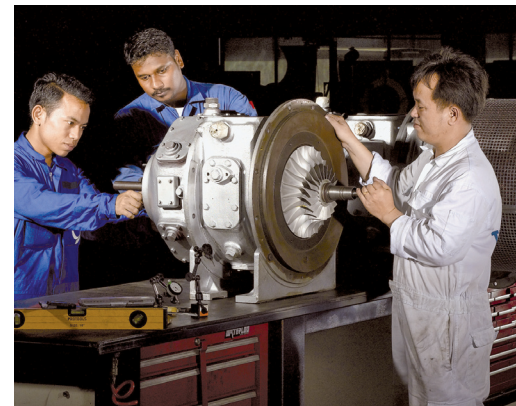
Tru-Marine fitters working on a turbocharger in Singapore
